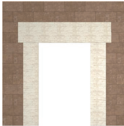
1-19 Post-and-lintel construction (John Burge).
